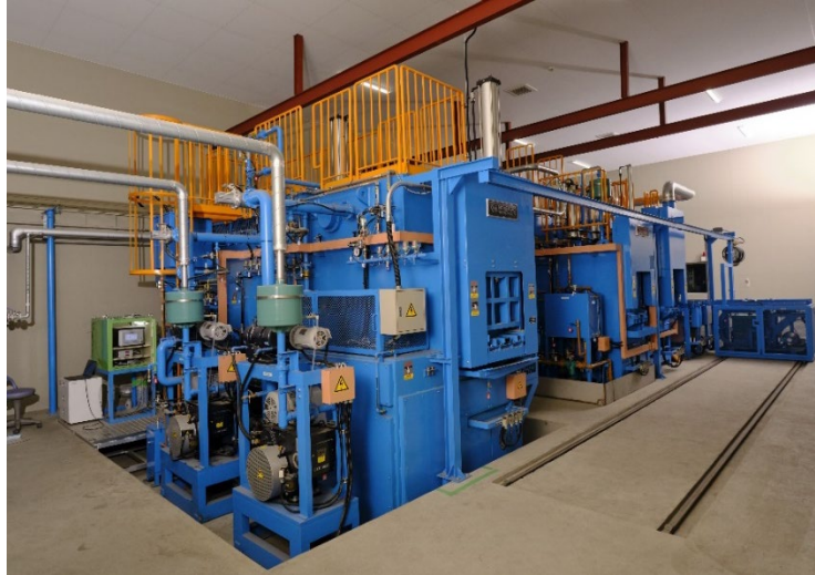
Carburizing furnace equipped with atmospheric pressure smart carburizing technology
