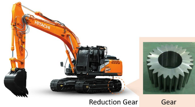
Gears incorporated in the reduction gear unit of a hydraulic excavator
